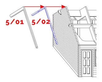
Barge boards need to be offset from the wall. Glue 5/02 pieces to the top edge of the angled gable. Make sure they are even and not protruding from the top edge. They can be very fiddly so take your time.
