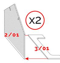
Begin the assembly by joining the side lower supports to the side walls. Make sure they are even and flush with the lower edge of the side wall.
