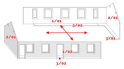
Fit another set of wall supports to the top edge of the walls. Ensure they are flush and even with top of the walls.
